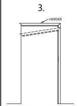
Install header into position approximately 1" from top and in the center of rough opening.
