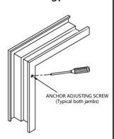
Tum adjusting screws in both jambs clockwise until anchor is resting against the wall. 6.
