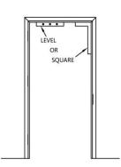
If feasible, hang door now and adjust frame on wall to allow proper door/frame clearance or plumb frame with carpenter square and/or level. (adjust header levelness by shiming under jambs.) 7.
