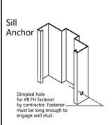
Check door opening dimension at base of frame (same dimension as between jambs at header.) Secure jambs with drywall screw (not furnished) through sill anchor at base of frame. Be sure to attach through both sill anchors on each side of jambs(4 places.)
